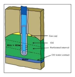
Figure 2: Oil and water segregation in "Static Condition
