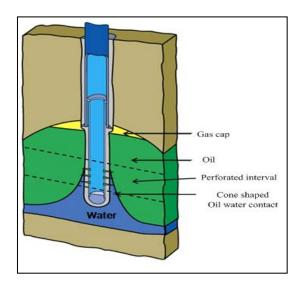
Figure 1: Water coning in "Dynamic Condition"
